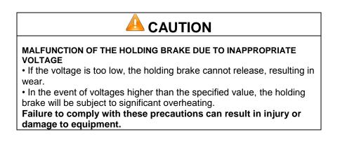
A motor with a holding brake needs a corresponding control logic which releases the holding brake at the start of the rotation movement, locking the motor shaft in time when the motor stops.
