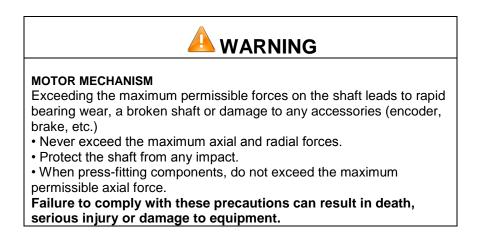
The maximum press-fit force is limited by the maximum permissible axial force on the ball bearings. This maximum axial force is stated in the motor technical data sheet.
